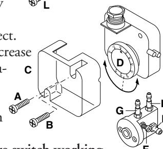
**Note:** The pressure measured at pressure port E must be within the limits of the pressure switch working range. If not, loose the locking nut of screw F and gradually turn the same: clockwise to reduce the pressure; counterclockwise to increase. At the end tighten the locking nut.
